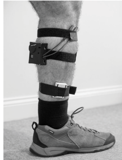
Figure 1: Image to show haptic device and vibrotactiles (without gait analysis markers in situ). The haptic device is the black box on the posterior calf. The vibrotactiles are shown positioned on the lateral aspect of the lower leg below the knee.
