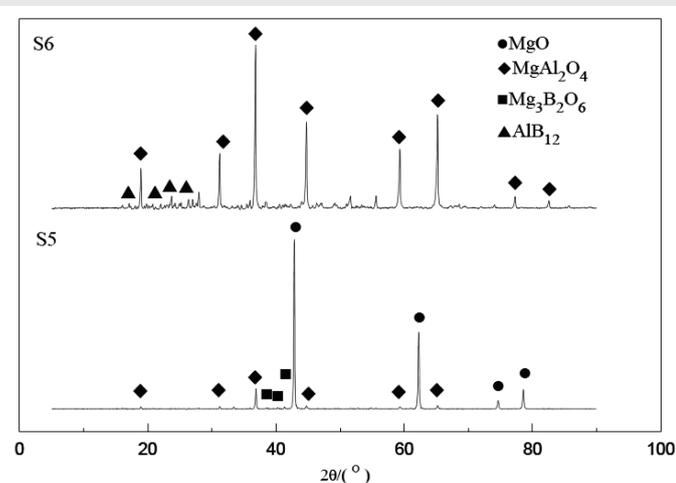
Figure 2: XRD patterns of fabrication  $\text{AlB}_{12}$  from Mg,  $\text{B}_2\text{O}_3$  and  $\text{Al}_2\text{O}_3$ .
