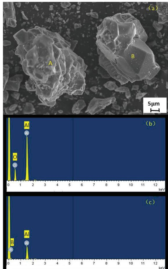
Figure 3: (a): Microstructure photographs of powder by SHS; (b): EDS analysis of A area; (c): EDS analysis of B area.
