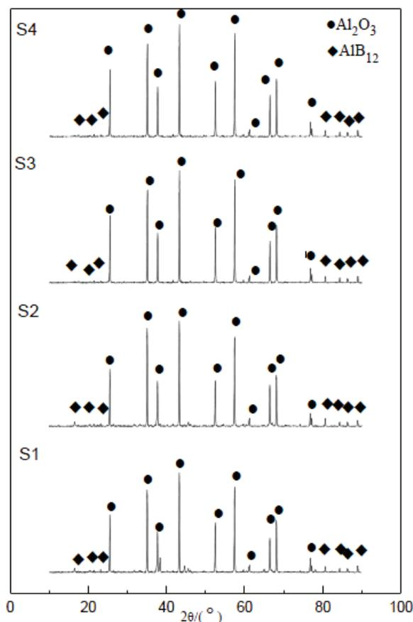
Figure 1: XRD patterns of fabrication AlB<sub>12</sub> from Al and B<sub>2</sub>O<sub>3</sub>.
