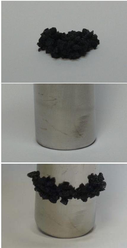
**Figure 2:** Magnetic attraction of hydrogel.
