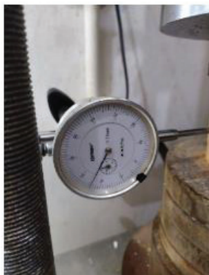
Figure 1: Strain Dial of Vesta Tester. The function of the strain dial is to measure the strain that occurs on the brick sample when it is given a certain amount of load.
