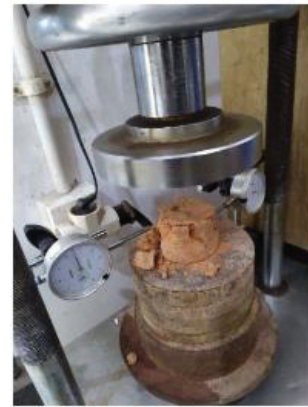
Figure 2: A sample of brick that began to crack when it is given a number of loads was calculated on how much strain occurs every 10 kN increments.
