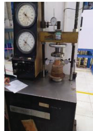
Figure 3: The Vesta Tester shows the amount of load applied to the bricks which being tested.
