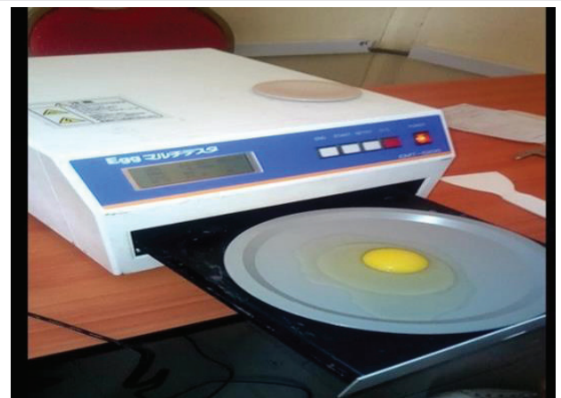
Figure 3: Measuring sample egg weight (g), albumen height (mm), yolk color score and Haugh unit (HU) by Egg multi tester (EMT-5200).
