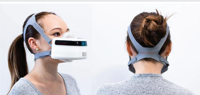
Figure 1: Wearable Breezing Pro™ metabolic tracker.
