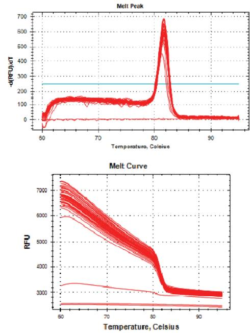
Figure 3: Melting peak and melting temperature of the gene 16SRNAr of *S. Heidelberg* used as reference gene.
