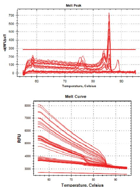
Figure 5: Melting peak and melting temperature of the gene *blaCTX-M2*.
